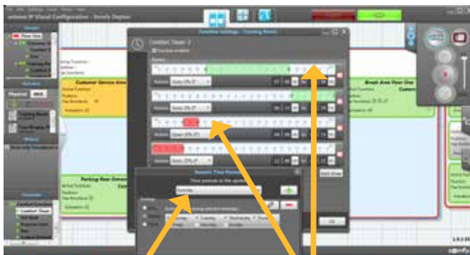
Choose from preset time periods to create customized timers Green means there are no conflicts, red means actions are overlapping
