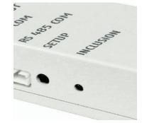
Press and hold the SETUP button for five (5) seconds to identify the ZBDMI in the network. Verify that the INCLUSION LED turns on within 10-15 seconds. When the LED is on, the ZBDMI is identified in the network.
